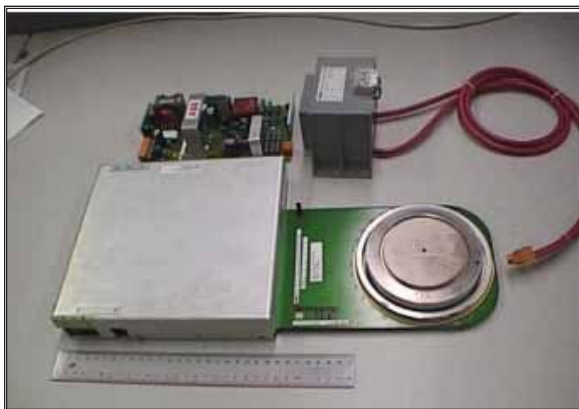
Figure 4. 4.5 kV 4 kV GCT, with power supply, & control power isolation transformer
