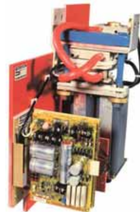
Figure 3. Water-Cooled GTO Module With Snubber, Capacitors, Gate Driver, And Devices
