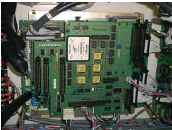
Figure 37. Modern MV PWM Single-board Control Processor
