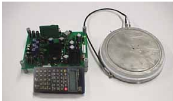
Figure 8. 4500 volt, 4000 amp IEGT and Firing Circuit
