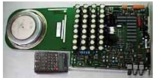
Figure 5. 4000 amp GCT, Integrated Control Box Components Exposed
